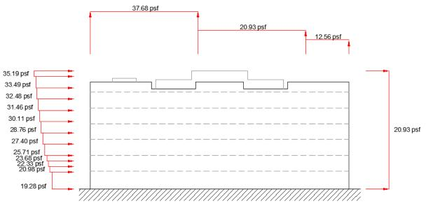
Figure 4.1, MWFRS East/West Wind Load Distribution
