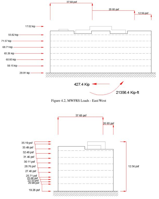
Figure 4.3, MWFRS North/South Wind Load Distribution
