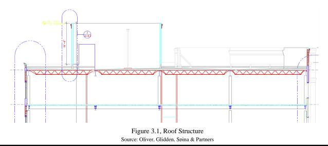
Rain and dead load was used to size the metal roof deck instead of recommended the roof live and dead load. The 27.89 lb/ft<sup>2</sup> rain load is greater than 20 lb/ft<sup>2</sup> live roof load. From the spot check, the original 1.5" thick metal roof deck spanning 5'-6" is sufficient to resist the superimposed rain and dead load.
