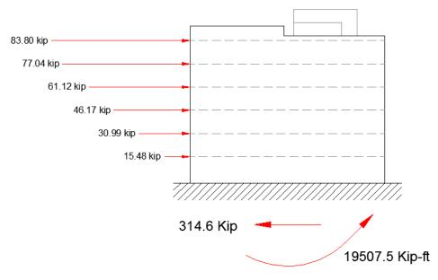
Figure 4.7, Seismic Loads Source: Oliver, Glidden, Spina & Partners
