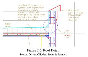
The insulated cast-in-place concrete was used in-lieu of rigid insulation with stone ballast. One reason is that the facility is in a hurricane zone. What it means is, loose material can potentially become airborne projectiles and cause damage when there is a hurricane. The insulated concrete has sufficient mass to resist becoming airborne. In addition, the added mass counters the uplift wind force.
